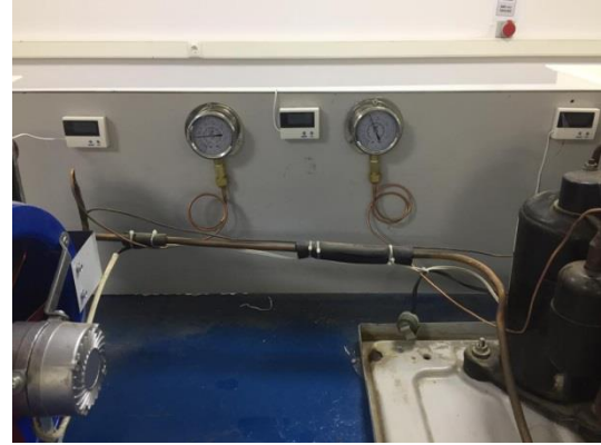
Figure 2. Secondary elements of heat pump system
